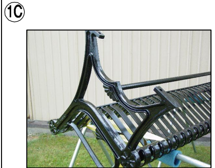
ATTACH CAST SUPPORT TO SEAT ASSEMBLY. IF HOLES IN CASTING DO NOT ALIGN WITH THE SEAT ASSEMBLY, ADJUST BY USING THE RATCHET STRAP.
